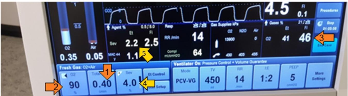
Newer anaesthetic machines with end-tidal control systems do this automatically where the anaesthetist chooses the oxygen and volatile anaesthetic percentages that they want the patient to receive and the anaesthetic machine automatically adjusts the fresh gas flow mix and vaporizer output to achieve this.
