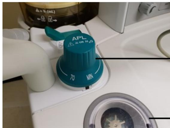
Note: Most GE anaesthetic machines with a bellows ventilator in the circle system bypass the reservoir bag and APL valve when using the ventilator.
